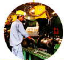
Automatic Cir-Seam Welding Process by Sub-Merged Arc Welding
