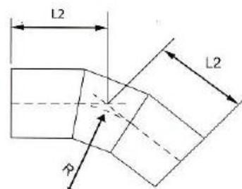
Figure 2. Gusseted bend type 2, over 30° up to 60°
