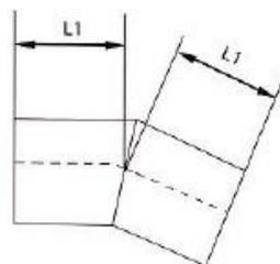
Figure 1. Gusseted bend type 1, not more than 30°
