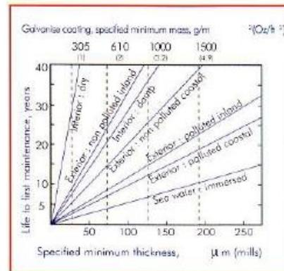
Eventhough steel is a strong material for fabrication of structural member, it still has to be protected from corrosion. There are many ways to protect it from corrosion but the most economical way is to coat with zinc using Hot Dip Galvanising (HDG) process. Generally, galvanising is carried out to conform to BS EN 1461:1999 (ISO) specifications.
