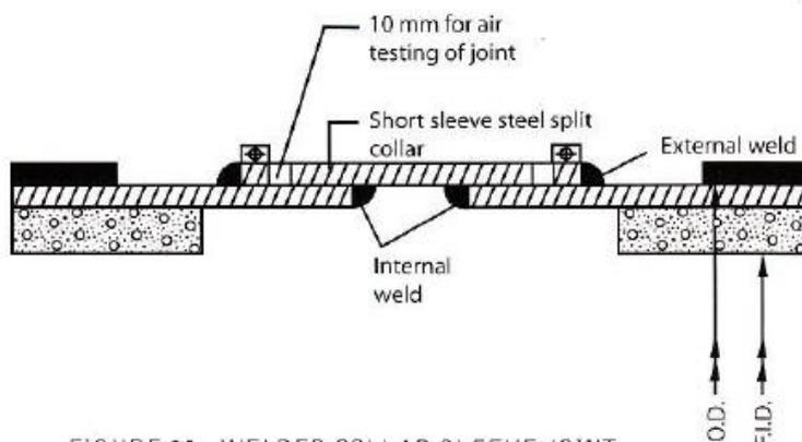
FIGURE 11 . WELDED COLLAR SLEEVE JOINT
