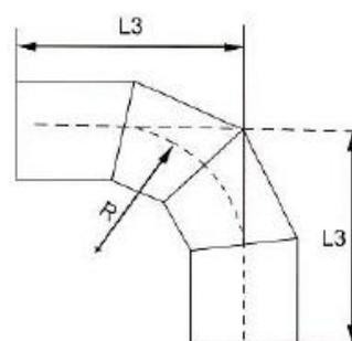
Figure 3. Gusseted bend type 3, over 60° up to 90°
