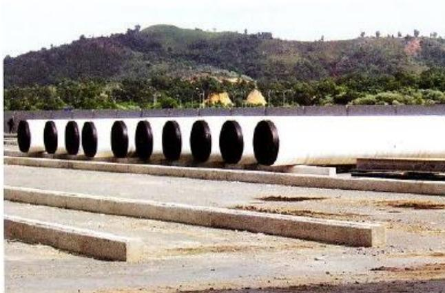
*Finished pipes for curing*
