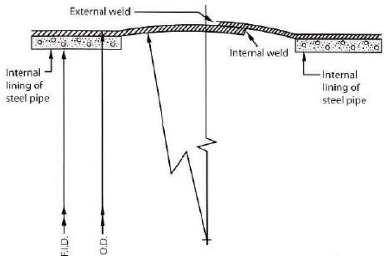
FIGURE 10 . SPHERICAL SPIGOT AND SOCKET JOINT
