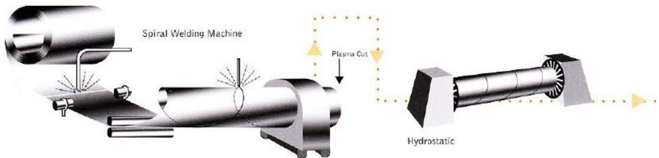
When compared to other alternatives, spiral welded steel pipes are stronger, higher-quality, more economical, and offer more design options for large diameter piping applications.
